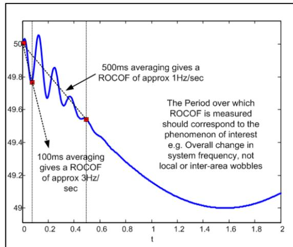
Figure 2: Effect of measurement window time on ROCOF value derived from a frequency signal.
