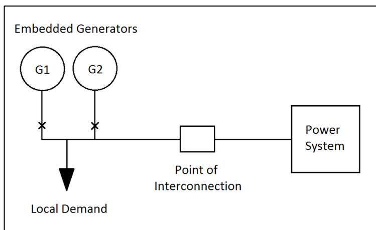
Figure 4: Typical configuration of distributed RES
