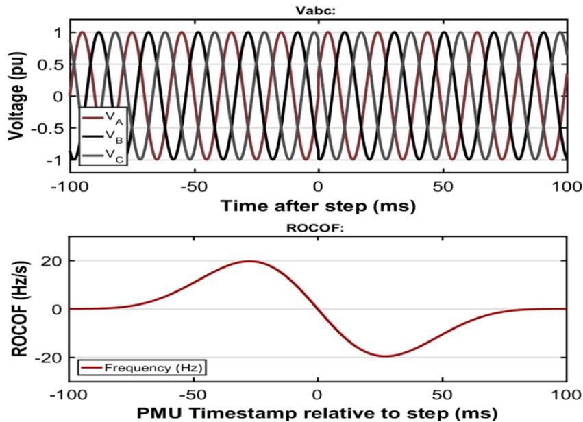
*Figure 8: Waveform (top) containing a 20-degree phase step at  $t = 0$  sec and its ROCOF perception (bottom)*
