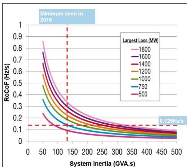
Figure 3: ROCOF experienced in GB for a range of inertia and loss of infeed events [1]
