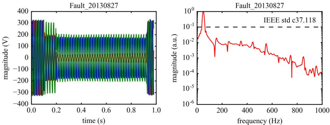
Figure 7: 3-phase voltage waveform (left) captured during a fault on the Glasgow distribution grid and its Fourier spectrum (right)
