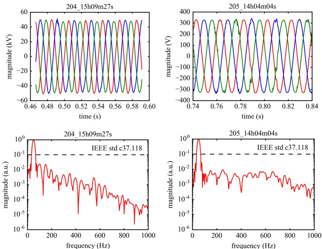
*Figure 6: Two typical 3-phase voltage waveforms (top) captured at the Bornholm distribution grid and their respective Fourier spectra (bottom)*
