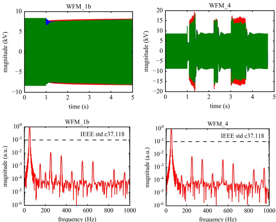
*Figure 5: Two 3-phase voltage waveforms (top) captured at the LiveLab 10 kV grid and their respective Fourier spectra (bottom)*
