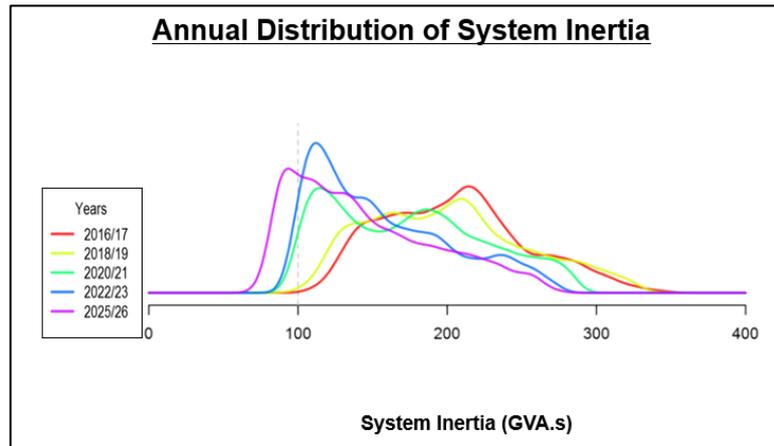
Figure 1: Projected probability density function of GB system inertia over an annual cycle [1]
